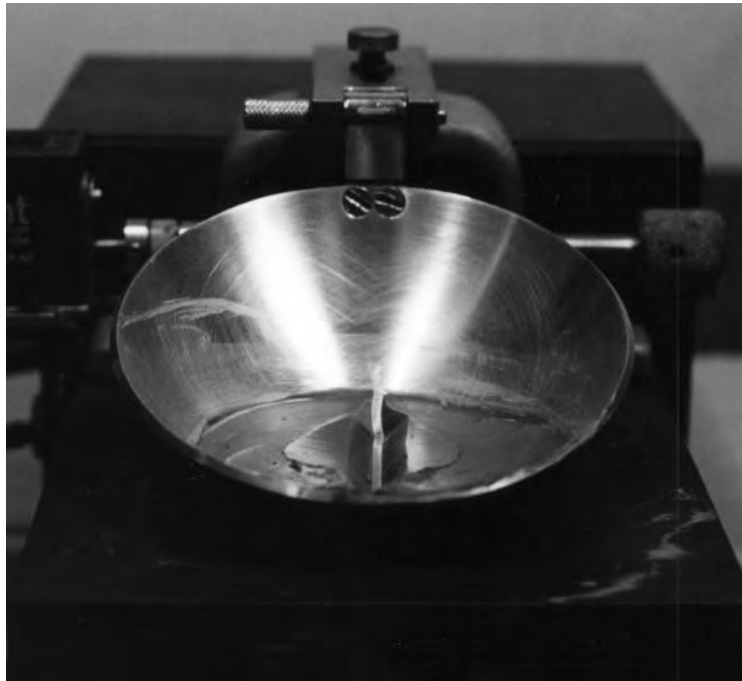
FIG. 7 Grooved Soil Pat in Liquid Limit Device
